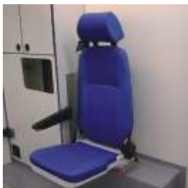
Seat, turnable on wheel arch, with integrated seatbelt
